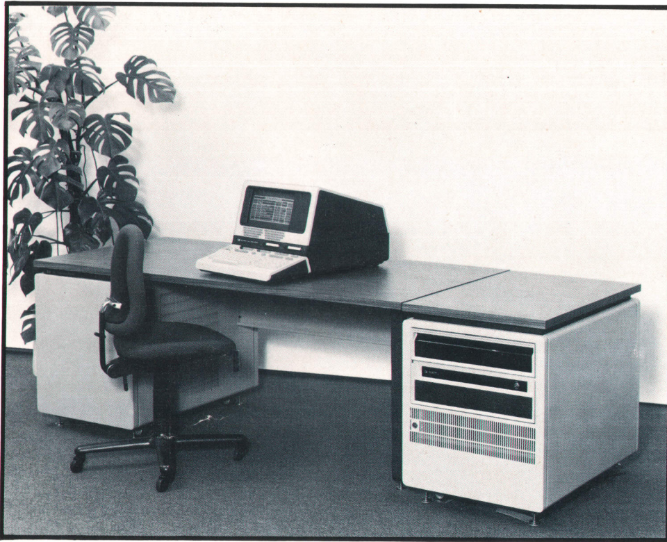
Fig. 1. HP 1000 Model 30 is intended for computational, automated test/measurement, or process control applications. RTE-II is the standard operating system (RTE-III optional). Model 31 is the same system in an upright cabinet.
